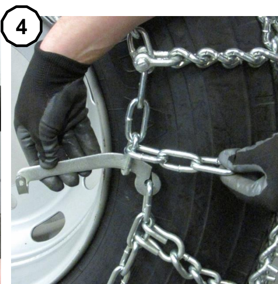
3 Take tension lever and pull it through a link in the side chain. If possible take back some links to get the chain tensioned well.
